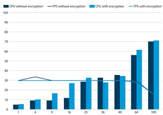
Smart Client performance measured on: Intel® CoreTM i7-8700K 3.7GHz CPU, 32GB memory, 2 X Nvidia GeForce GTX 1080 Graphics cards, Microsoft Windows 10 Enterprise OS.
